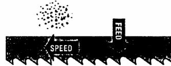
Burned heavy chips – reduce feed rate and/or band speed.
